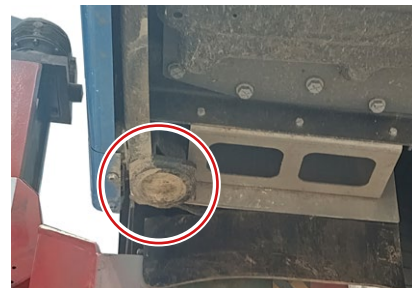
Rear RHS Jacking Point.
