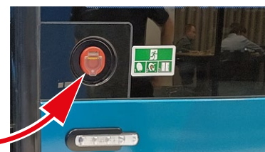
External Emergency Exit Button
