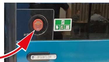
External Emergency Exit Button
