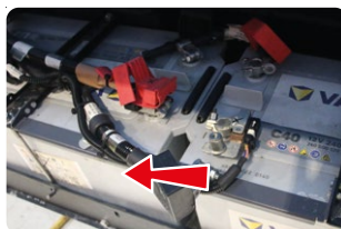
The 24v Battery Disconnect switch is at the rear of the battery compartment.
