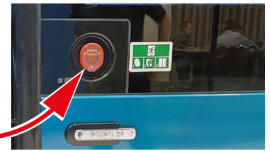
External Emergency Exit Button
