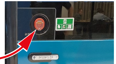
External Emergency Exit Button
