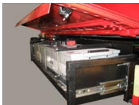
Vehicle 24V DC Battery tray extended
