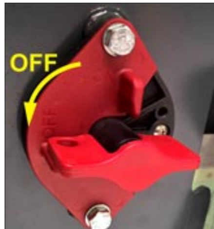
Master Disconnect Switch
