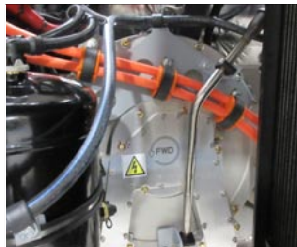
Direct Drive Traction Motor (DDTM) installed
