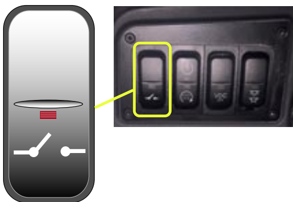
Master Switch on Drivers Dashboard
