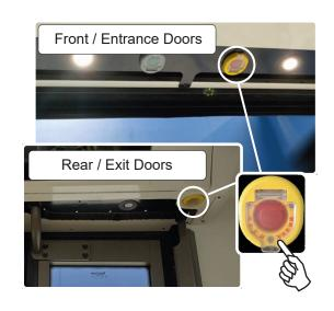
If the doors do not operate they can be pushed open manually.
