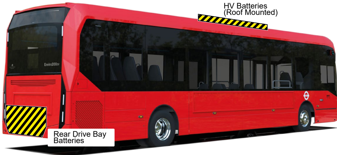
Rear Drive Bay Batteries
